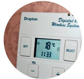
Some modern heating controls now combine a heating timer and the thermostat, allowing you to set different temperatures for different times of the day.
